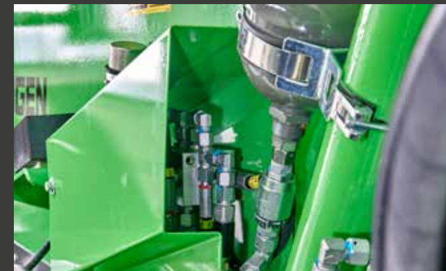
4 Important valves and electrics are protected and accessible from the outside, even when the telescopic boom is lowered.
