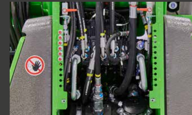
6 Best possible access to the main manifold, hydraulic oil tank and return filter.
