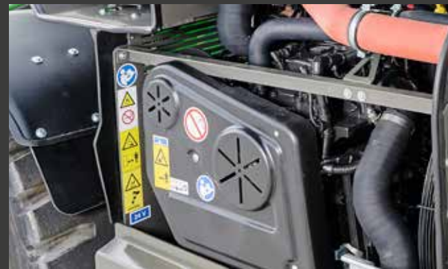
1 All service points easy to access thanks to transversely mounted engine.
