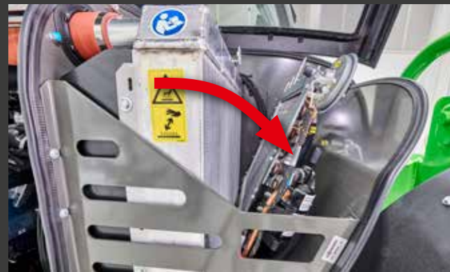
2 Very good access to the cooler thanks to the folding air conditioning condenser.
